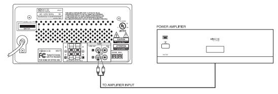
connected Axcess to the external amplifier, Axcess' volume control will control the volume of the amplifier and the speakers connected to it.
