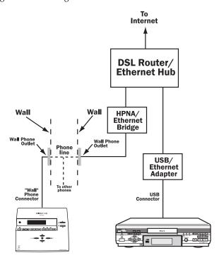
The following HPNA/Ethernet bridge models are verified by Kenwood to work with Axcess and Entré:
