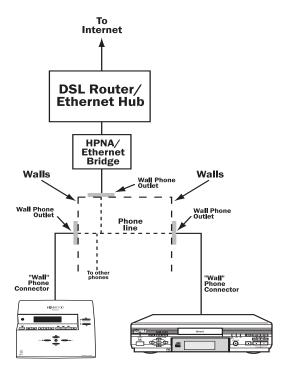
If you use a broadband Internet connection and you connect Entré to the Internet via a Universal Serial Bus (USB)/Ethernet adaptor *and* an HPNA/Ethernet bridge, you will be able to use all of Axcess' functions including Internet Radio. Connect the components according to the following illustration:
